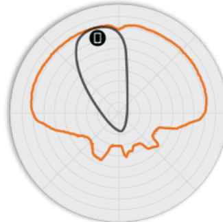
Figure 4. H320 2.4GHz Elevation Antenna Patterns
