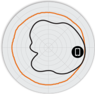
Figure 2. H320 2.4GHz Azimuth Antenna Patterns
