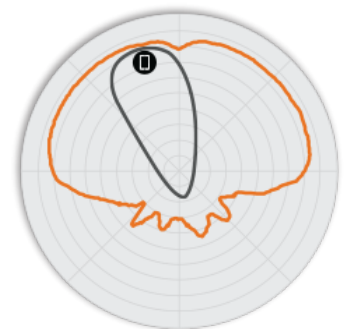
Figure 5. H510 5GHz Elevation Antenna Patterns
