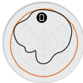
Figure 3. H510 5GHz Azimuth Antenna Patterns
